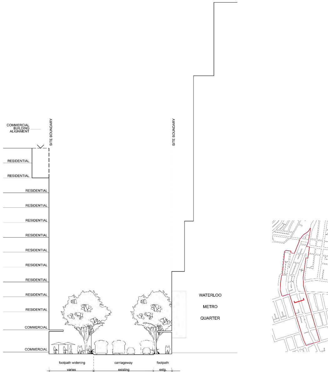
Figure 95 Street Cross Section - Botany Road (North)
